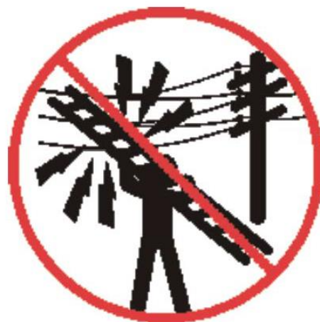
Beware of electrical hazards when transporting ladder
